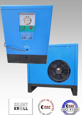
The "refrigerated" type dryer, to purify compressed air equipment, serves to eliminate the humidity that occurs at the outlet of the compressor, due to the temperature of the aspirated air. This humidity occurs because at the exit of the compressor the air is at its level of water vapor saturation. To prevent its use in these conditions damage the installation and equipment, it must be dried.
