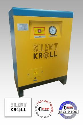
The "refrigerated" type dryer, to purify compressed air equipment, serves to eliminate the humidity that occurs at the outlet of the compressor, due to the temperature of the aspirated air. This humidity occurs because at the exit of the compressor the air is at its level of water vapor saturation. To prevent its use in these conditions damage the installation and equipment, it must be dried.
